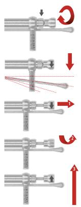
To dismantle the torque wrench for cleaning procedure, unscrew the wheel and then remove the inner bar where the spring is assembled.
